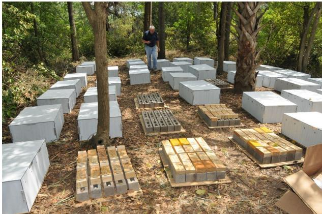
Figure 35. Large scale test box installation. Each test unit will be covered with a grey cover.
