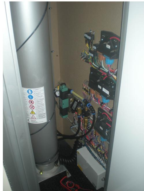
Figure 24. Antenna cylinder and cylinder stop sensor bracket in the Homeland Security Emergency Preparedness bus.
