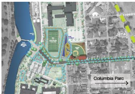
St. Bernard Neighborhood Campus | new bayou crossing, water plaza and playground, green streets, and athletic fields that double as retention basins connect neighborhood and institutions Source: Waggoner & Ball Consultant Team
