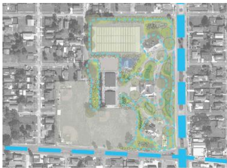
Milne Campus | open land and athletic fields are connected to the city's drainage network to provide 81 acre feet of storage capacity Source: Waggoner & Ball Consultant Team
