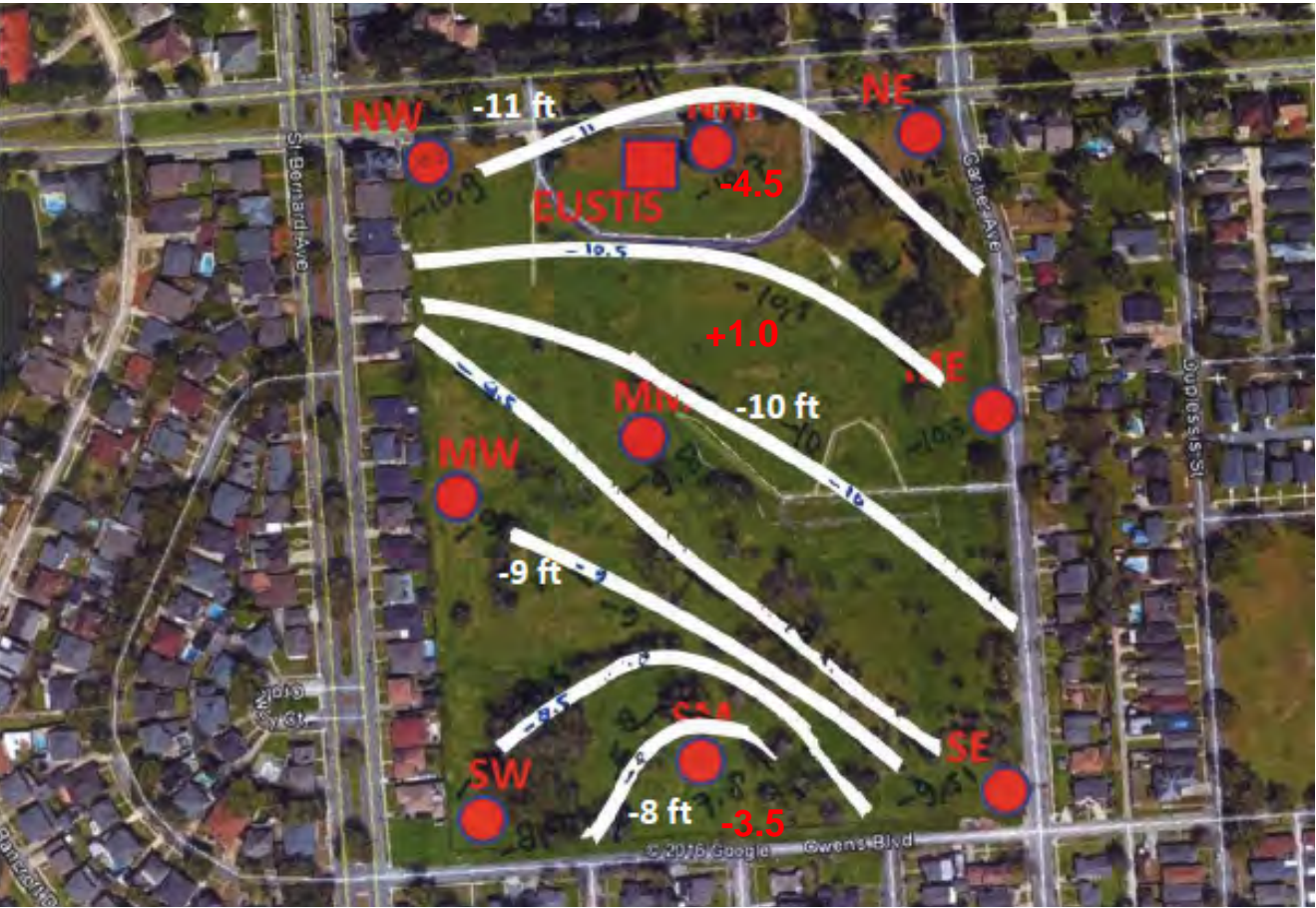
GROUNDWATER MONITORING NETWORK & WATER LEVEL CONTOURS IN FEET BELOW SEA LEVEL
