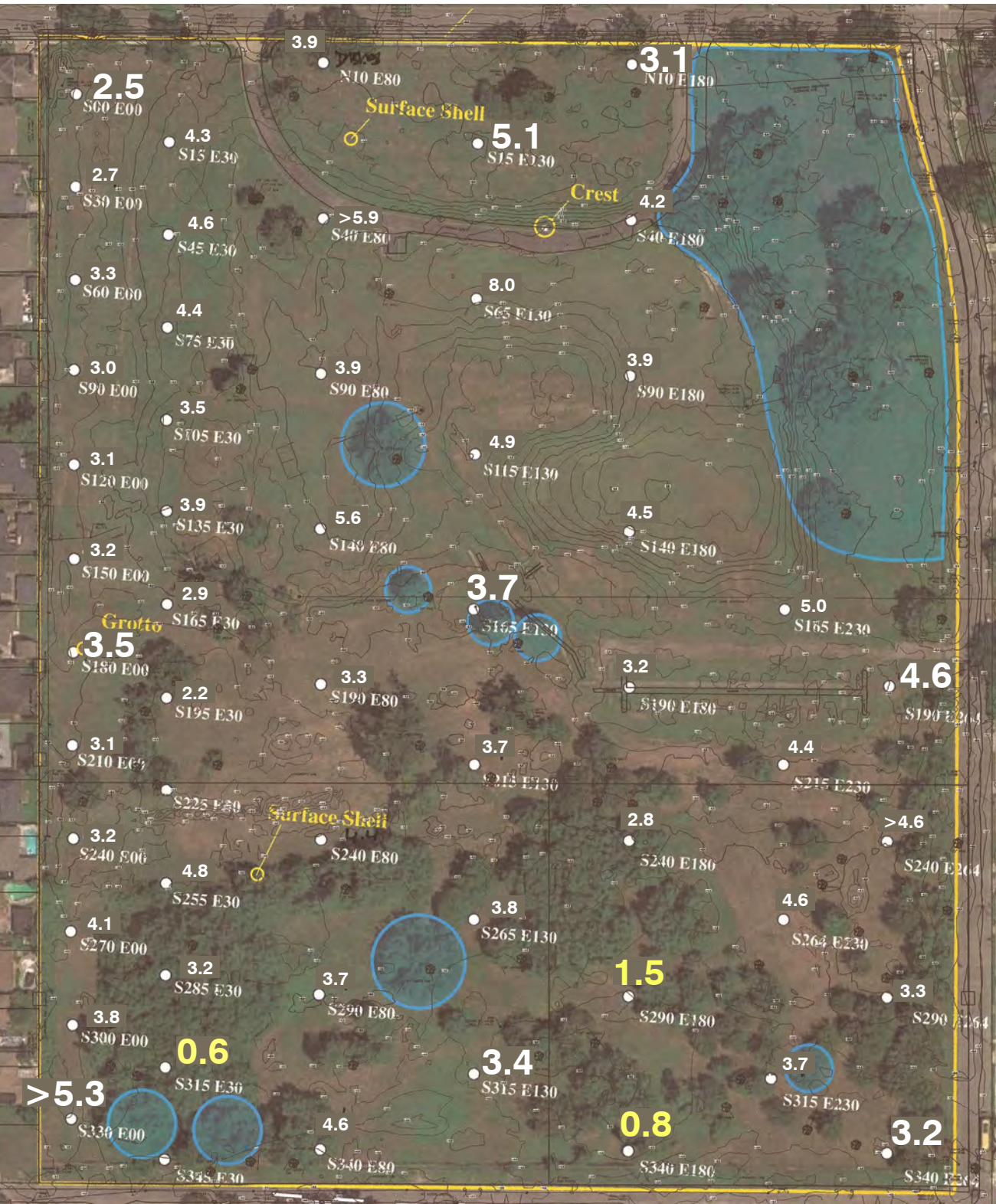
CLAY LAYER THICKNESS (FEET) BASED ON FEMA'S ARCHAEOLOGICAL SOIL ASSESSMENT
