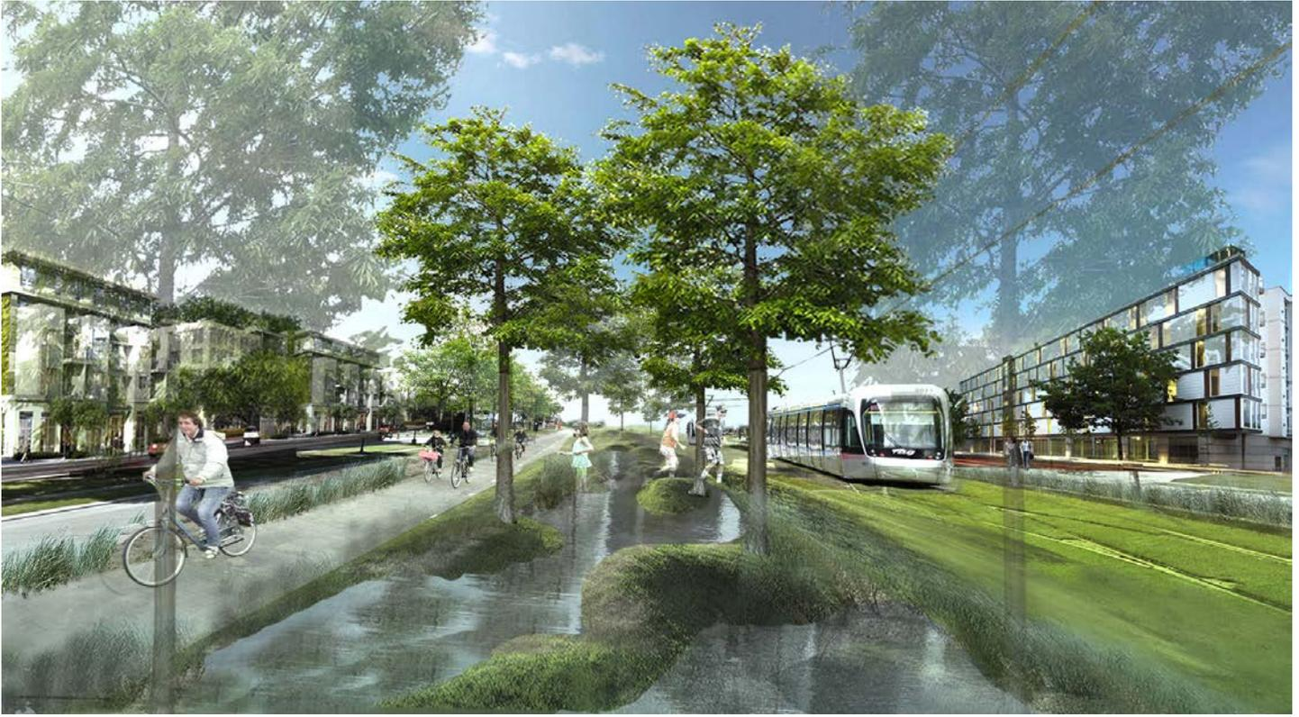
Wet Condition | Wide neutral ground (median) of Elysian Fields Avenue, reshaped to hold and filter stormwater
