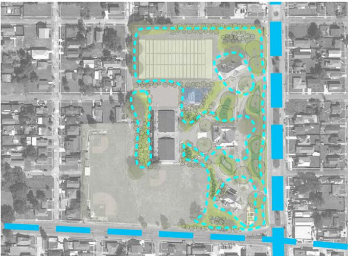
Milne Campus | open land and athletic fields are connected to the city's drainage network to provide 81 acre feet of storage capacity
