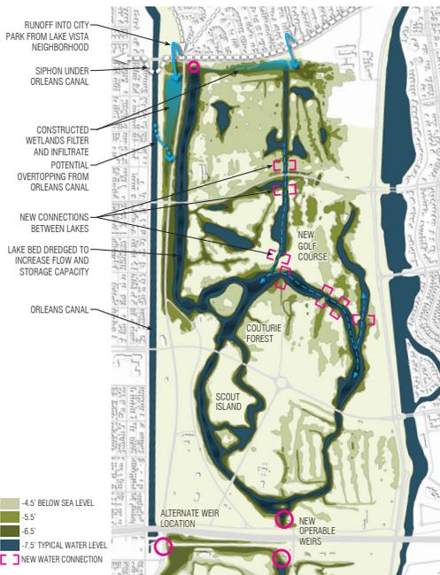
**Diverting Runoff |** redirection of runoff from lakeside neighborhoods into park for retention and filtration, reducing flood risk and pumping
