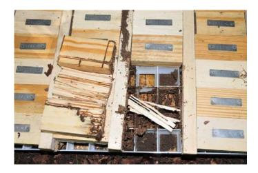
**Figure 27.** FST damage to wood blocks in a pilot test box.
