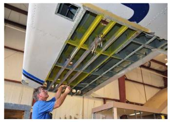
**Figure 2.** Ben Smith repairs corrosion on the airplane wing.
