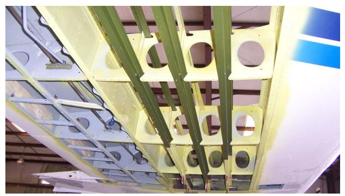
Figure 21. The right wing of the Britten-Norman Islander after remediation of corrosion.
