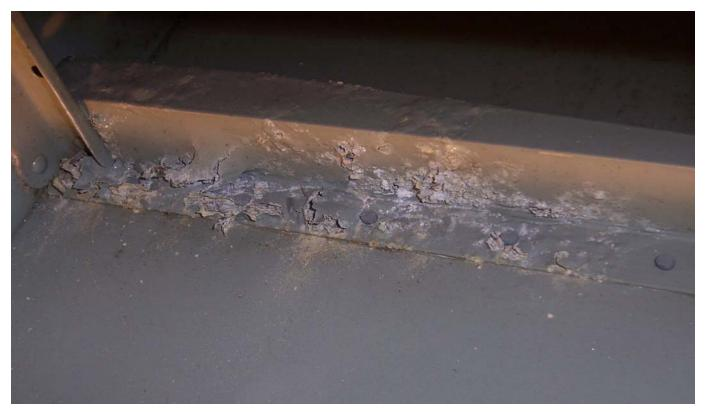
Figure 20. Extensive corrosion was found in the Britten-Norman Islander spray aircraft.
