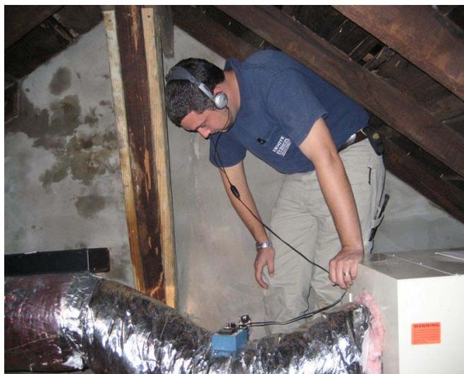
**Fig. #11:** Dr. Kenneth Brown uses an acoustic detection device to locate Formosan subterranean termites.
