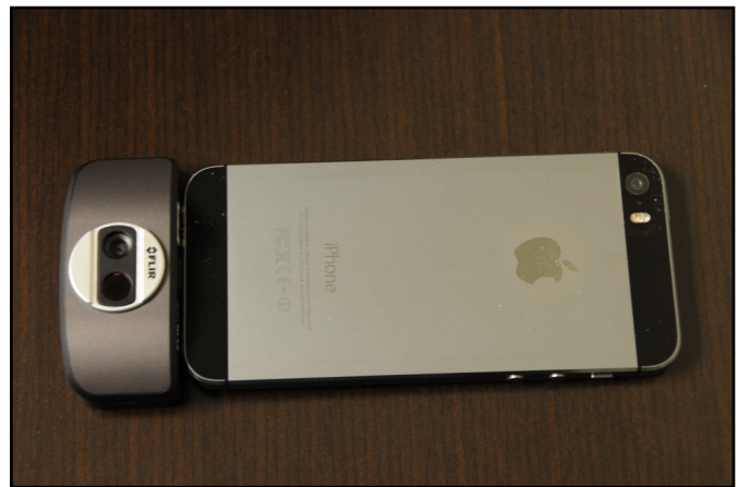
Figure 38. Camera side of the FLIR ONE infrared camera attached to a smartphone.
