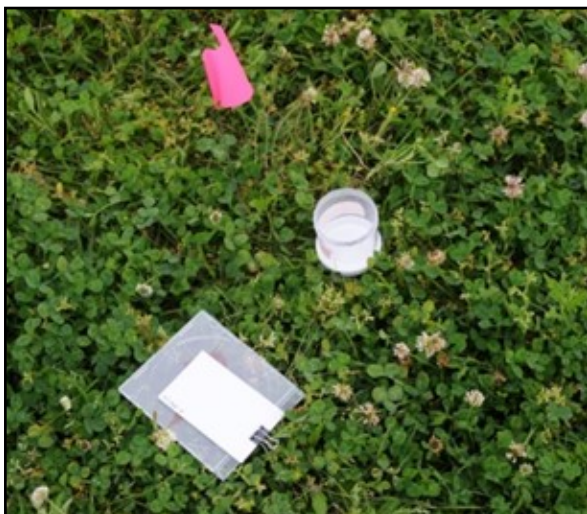
Figure 19. Open field trial set-up with flag marking location, bio-assay collection cup and card for collecting droplets.
