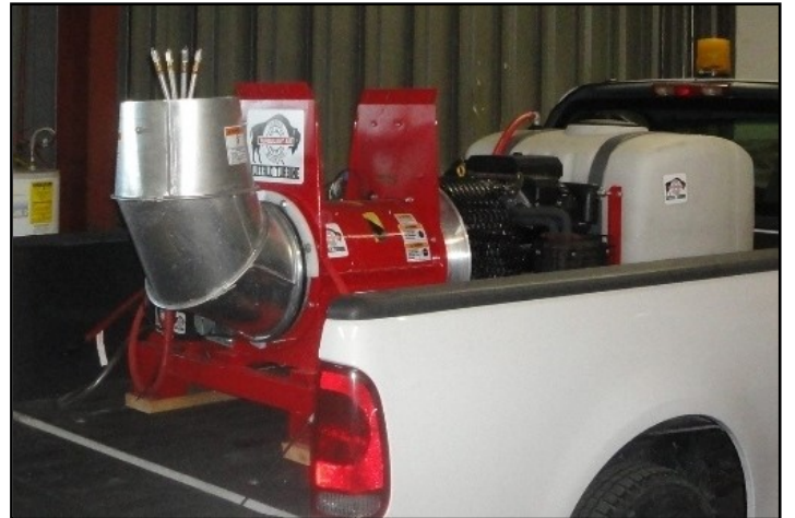
Figure 28. The Buffalo Turbine CSM/3 was adapted for mosquito control.
