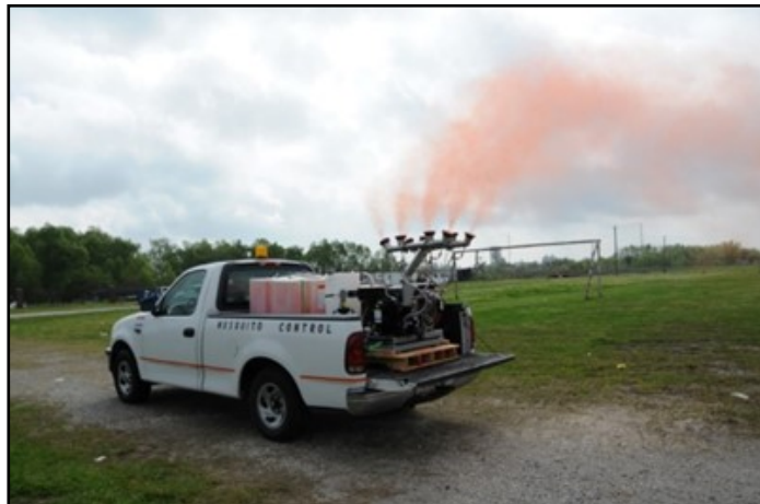
Figure 18. The Curtis-Dynafof LV-8 adapted for a mosquito control application, using dyed material in an open field trial.
