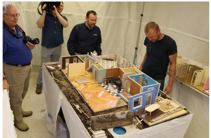
Figure 48. Tear down of the Tiny Termite House revealing complete loss due to termite damage.
