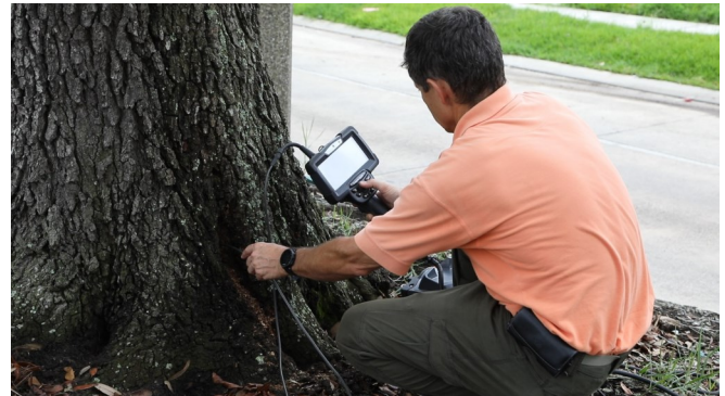
Figure 56. Using a flexible fiber optic borescope to determine termite activity and extent of termite damage.
