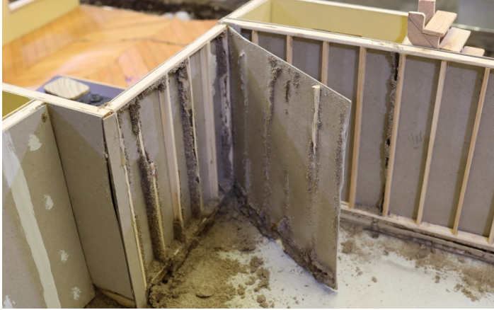
Figure 49. Formosan subterranean termite damage to interior wall studs in the Tiny Termite House. Note how only some studs were damaged and got covered with mud.
