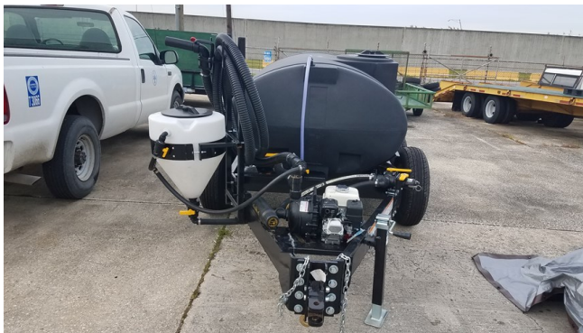
Figure A2-7. A 500-gallon nurse tank was purchased to mix the larvicide and to reload the A1 Mist Sprayer while in the field.
