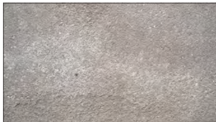
Granite – A hard rock, consisting of small, yet visible, grains of minerals, which can be highly polished or textured; used for walls, piers and street curbs; commonly in gray, black and pink.
