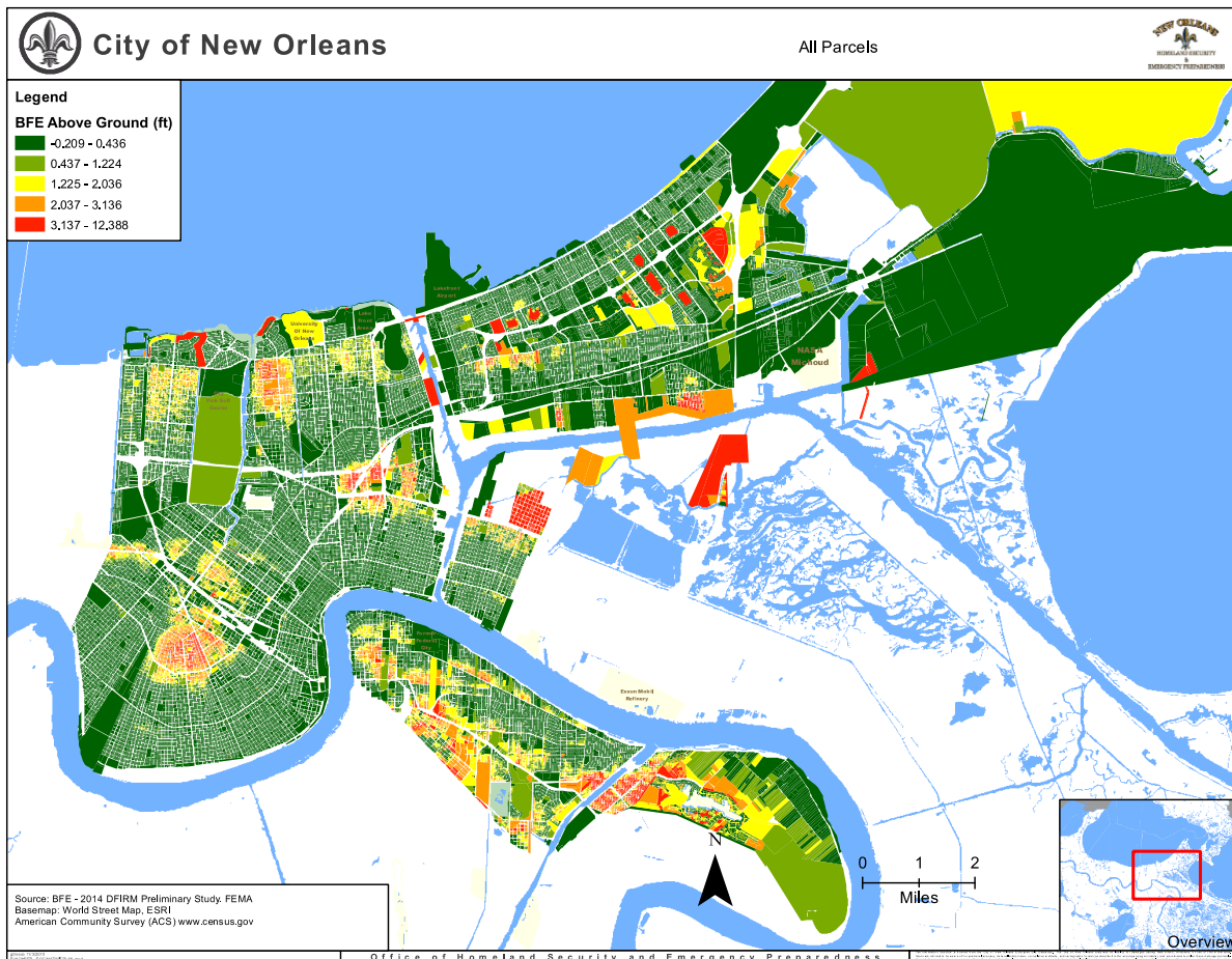
Figure 6-1 Topography of New Orleans Showing Base Flood Elevation Above Ground – All Parcels
