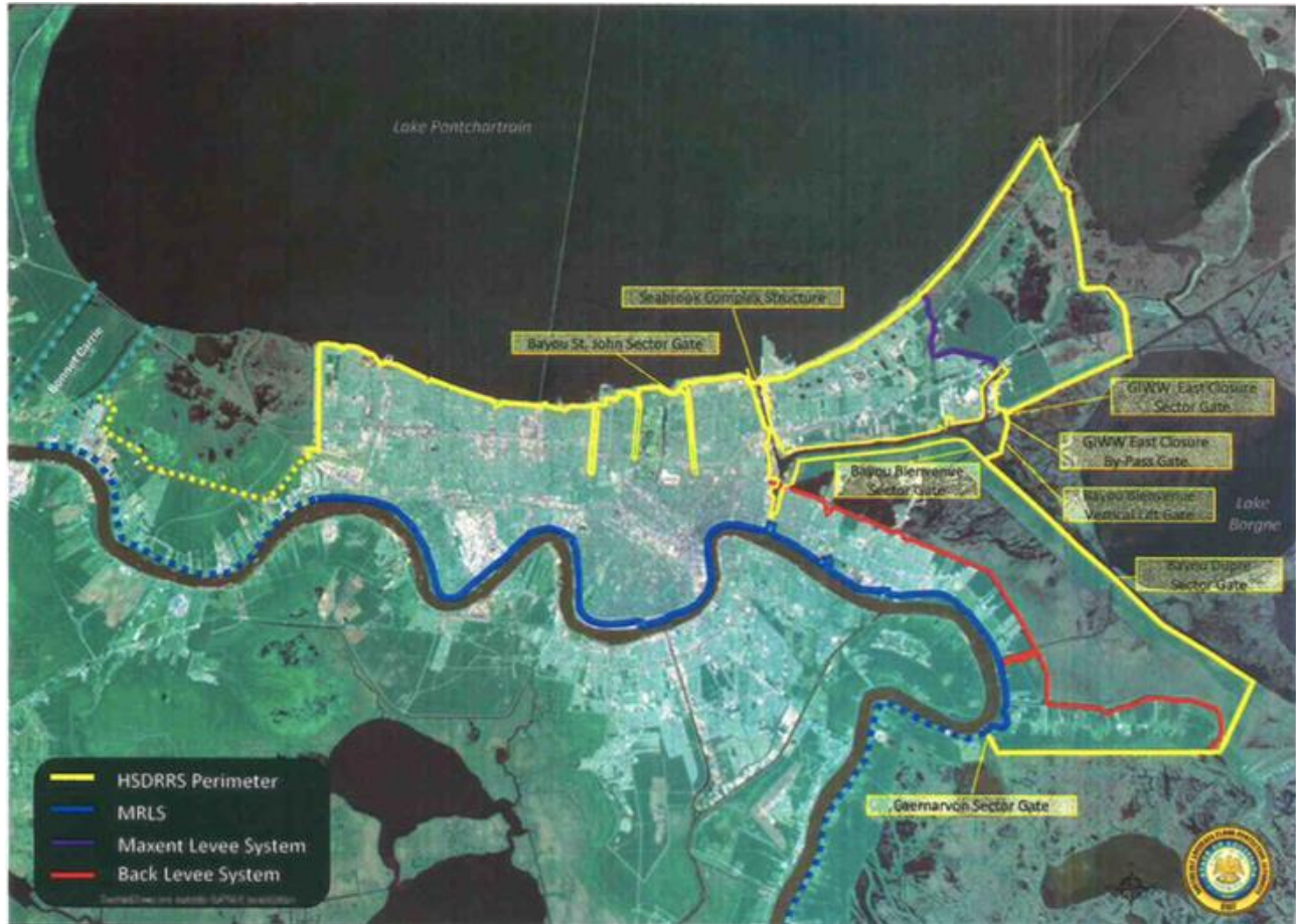
Figure 6-23 Orleans East Bank Levee Protection System
